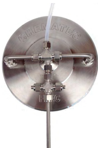
B Vent tube fitted for flow check
