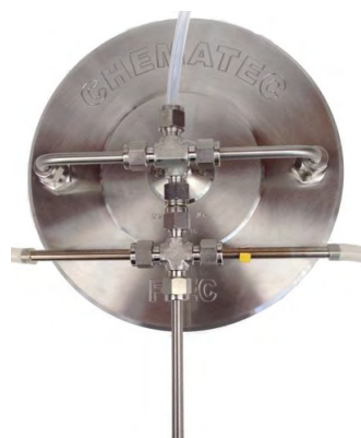
D Spacer replaced by the vent tube
