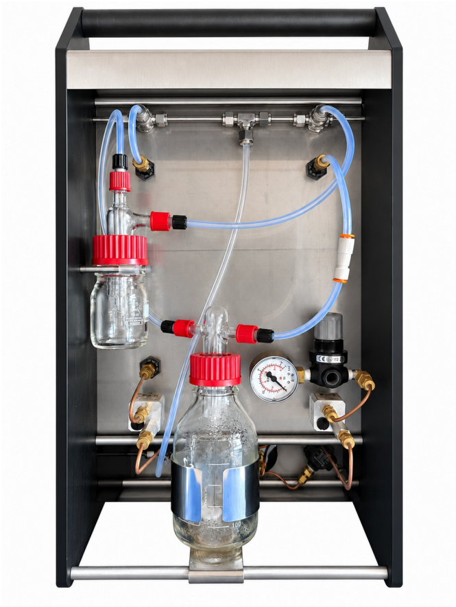
Figure 3. FL-1000 rear configuration with a condensate bottle and rear regulator.
